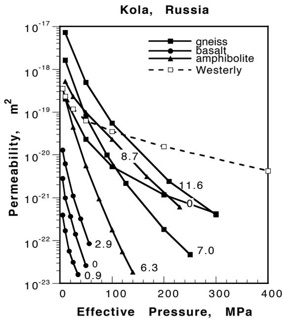
Figure 2. Permeability of core samples from the Kola well in Russia. Numbers indicate sample depth in km. Westerly granite (Brace *et al.*, 1968) included for comparison.
