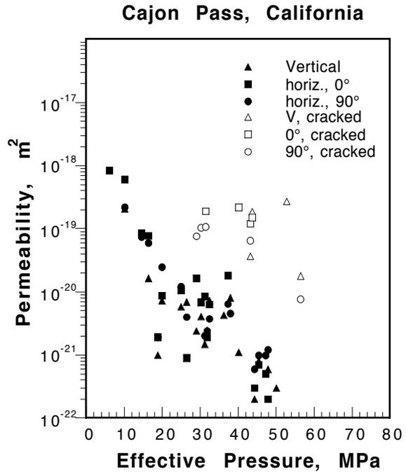
Figure 1. Permeability of intact (closed symbols) and fractured (open symbols) crystalline rock samples from the Cajon Pass drillhole in California under estimated *in situ* effective pressure conditions. Measurements in three mutually perpendicular orientations show the extent of permeability anisotropy.
