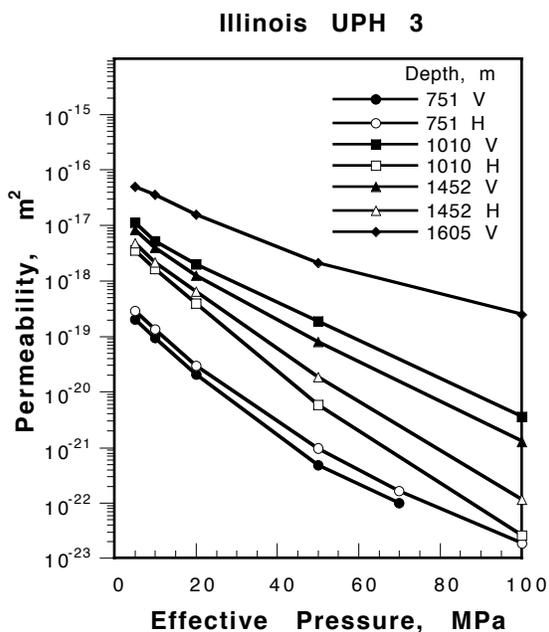
Figure 4. Permeability of granite core samples from the Illinois UPH 3 drillhole. Sample depth in meters for vertical (V) and horizontal (H) cores.
