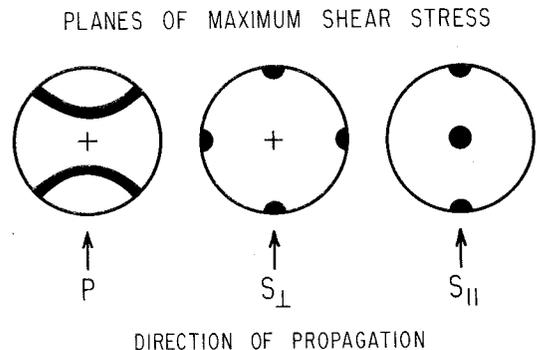
Fig. 4. Equal-area projection of poles of maximum shear planes caused by the passage of  $P$ ,  $S_{\perp}$ , and  $S_{\parallel}$  waves. The direction of wave propagation is indicated by the arrows. The axis of the sample is located at the center of each plot. The poles of vertical cracks would fall along the rim, whereas horizontal cracks would be located at the center of each plot.
