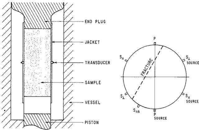
Fig. 1. Schematic view of sample mounted in pressure vessel and cross section of sample showing location of transducers and trace of fracture surface.
