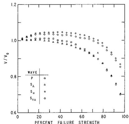
Fig. 2. Velocity relative to velocity at hydrostatic pressure for  $P$ ,  $S_{I}$ ,  $S_{II}$ , and  $S_{IIA}$  waves.
