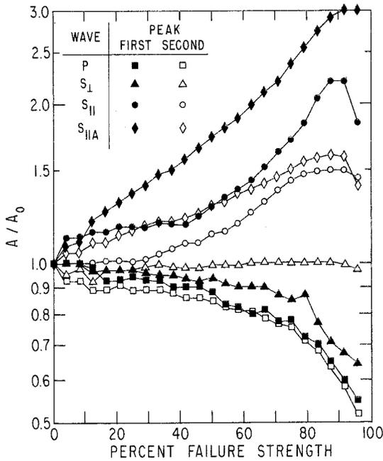
Fig. 3. Amplitude ratios for first and second peaks of  $P$ ,  $S_{\perp}$ ,  $S_{\parallel}$ , and  $S_{\parallel A}$  waves as a function of failure strength.  $A_0$  is the amplitude of the appropriate peak at hydrostatic pressure.
