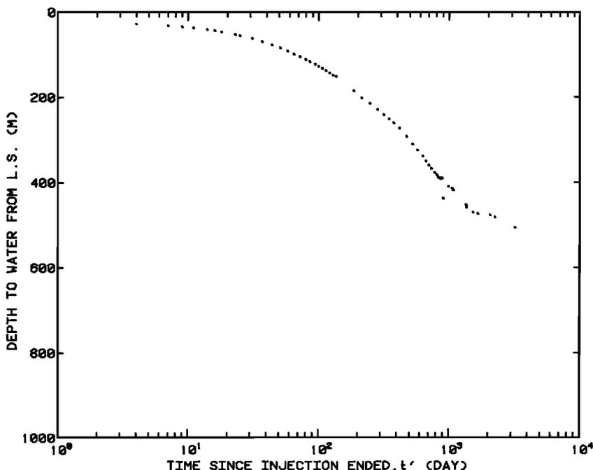
Fig. 6. Observed water levels in the RMA disposal well since injection ended.
