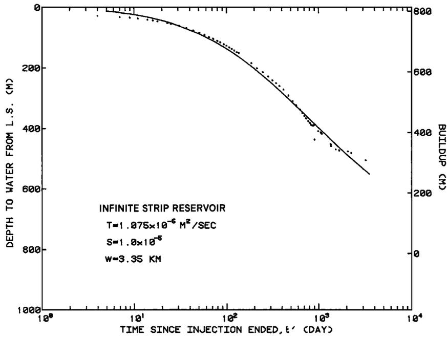
Fig. 8. Comparison of computed and observed water levels following injection in the RMA well—best fit for the infinite strip reservoir model.
