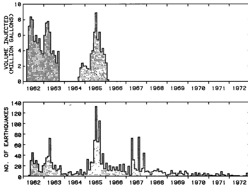
Fig. 1. Comparison of fluid injected and the frequency of earthquakes at the Rocky Mountain Arsenal. Upper graph shows monthly volume of fluid waste injected in the disposal well. Lower graph shows number of earthquakes per month. The apparent correlation for the period 1962-1966 was first noted by Evans [1966].
