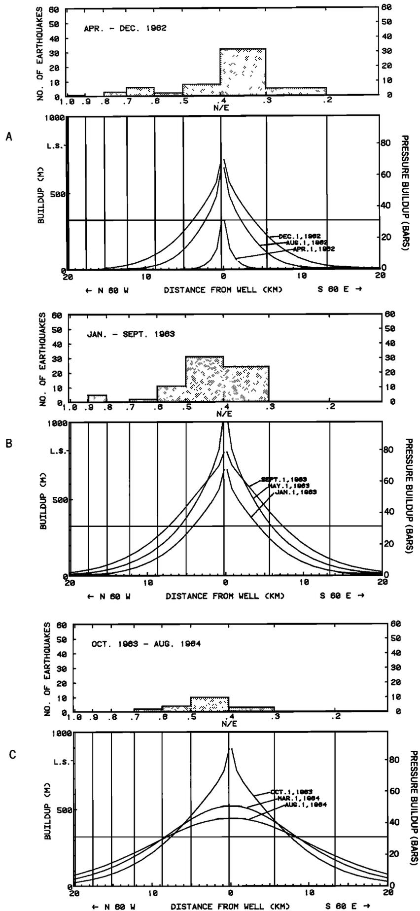
Fig. 14. Comparisons of earthquake distribution with computed pressure buildup in the Precambrian reservoir for nine characteristic periods.
