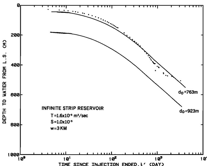
Fig. 7. Comparison of computed and observed water levels following injection in the RMA well—first trial for infinite strip model.
