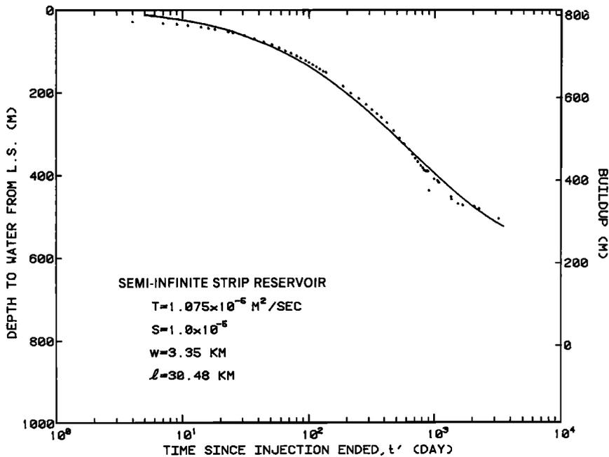
Fig. 9. Comparison of computed and observed water levels following injection in the RMA well—best fit for the semi-infinite strip reservoir model.
