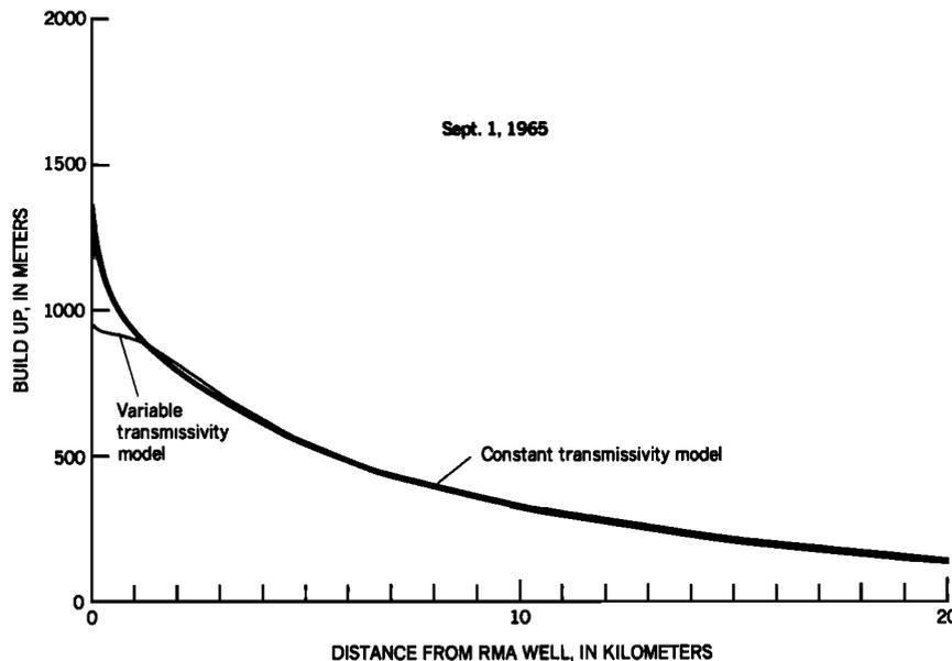
Fig. 15. Comparison of hydraulic head buildup computed by constant transmissivity model and variable transmissivity model. The variable transmissivity model simulates the effect of rapid fluid flow in fractures opened by high pressure.
