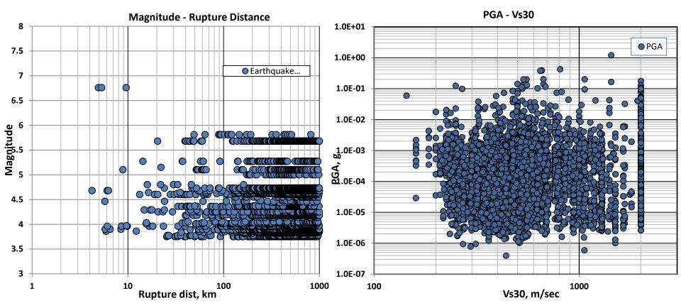
Data in the database are sparse and cover mostly a limited range of moment magnitudes **M**<6.0 with only three data points with **M**>6 from the 1985 **M**=6.8 Nahanni earthquakes.
