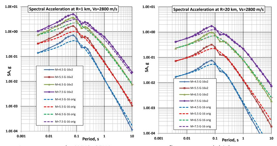
In contrast to the WUS, CENA response spectra flatten at much higher frequencies. In G-16 and G-16v2 models response spectra flatten completely at a frequency of 250 Hz and this corresponds to the value of PGA.
