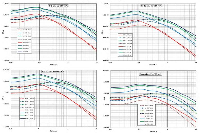
At fault distances up to about 100 km long period components of response spectra are similar in the East and West. At larger distances eastern data are higher at all periods due to higher Qsa.
