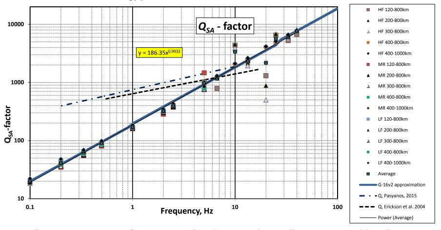
In a frequency range of 0.1-40 Hz the data can be well represented by the power law with the average dependence of:
