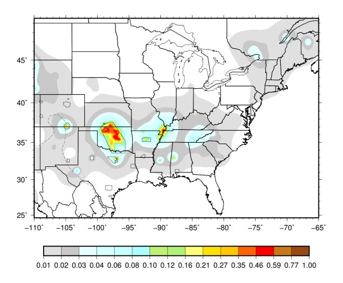
Peak acceleration, expressed as a fraction of standard gravity (g) for 1% probability of exceedance in one year and Vs30 site condition of 760 meters per second
